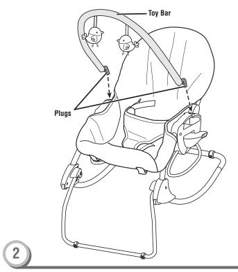
• Fit the plugs on each end of the toy bar into the sockets in each side rail.
